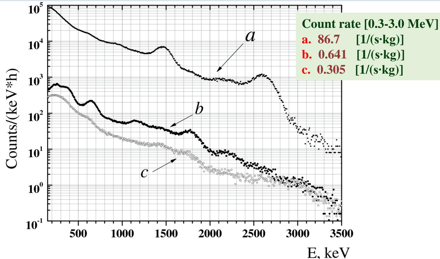
Background spectra in the unshielded room of DULB (a), in a low-background box (b), in a low-background box with additional 15 cm Pb shield(c).
