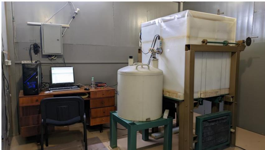
Low-background shield is consists of: 80 mm of polyethylene, 1 mm of cadmium (Cd), 150 mm of lead (Pb) and 180 mm of copper (Cu)
