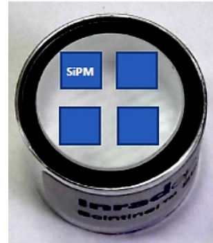
Detection of scintillation photons with four SiPMs 6×6 mm 2 , SensL, J ser.
