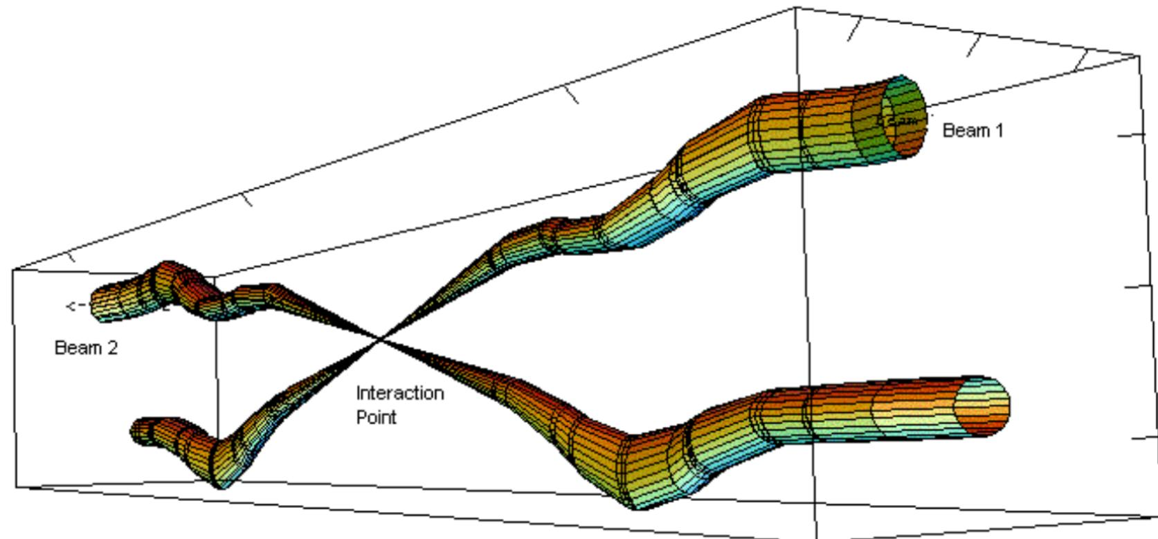
Relative beam sizes around Interaction Point 1 (IP1) ATLAS in collision
